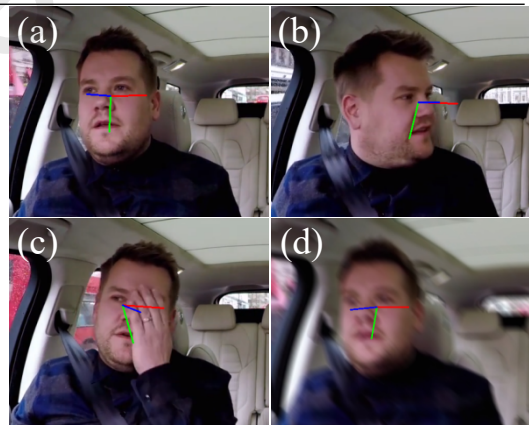
Fig. 1. Head pose estimation by the proposed method. (a) Normal driving. (b) Talking in driving. (c) Occlusion by hand in driving. (d) Bumps in fast driving. Three color lines denotes the three angle directions of human head pose.
